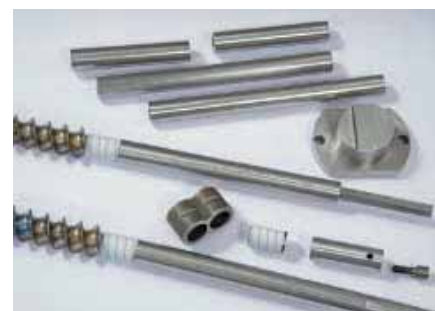
Fig 3: Adjustable screw length and flexible configurations to change residence time and processing conditions.
