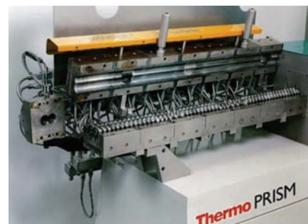
Figure 1: PRISM 36:1 extruder showing open, horizontally split barrel for easy cleaning and inspection.
