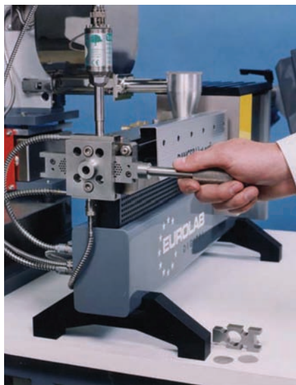
Figure 3: PRISM EuroLab TSE, showing screen changer for Delta P pressure test
