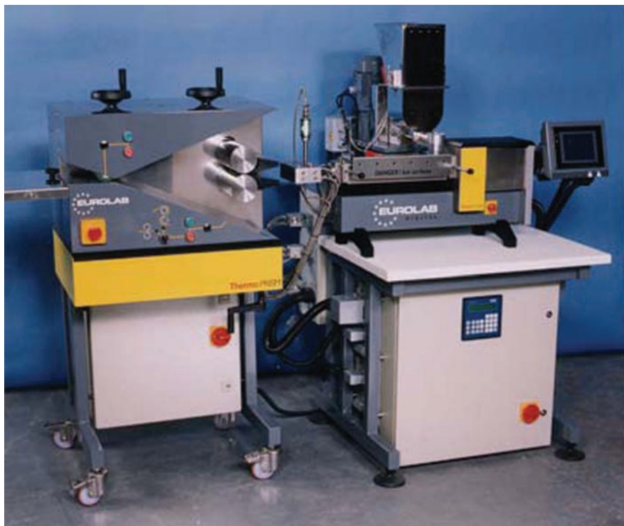
Figure 2: PRISM EuroLab featuring sheet line take-off system
