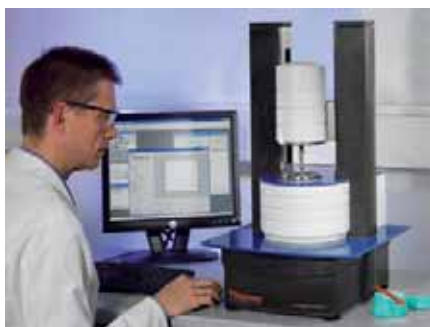
Fig. 2: HAAKE RheoStress 1 with built-in Peltier temperature control unit for plate and cone measuring geometries
