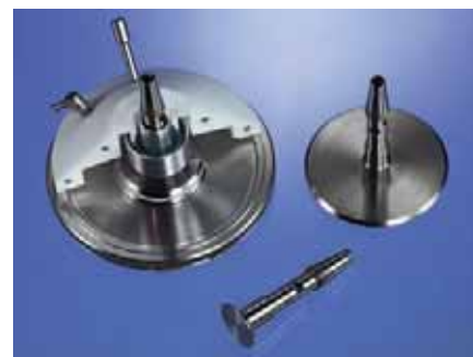
Fig. 4: Titanium geometry with measuring plate cover (MPC) with same diameter for optimised gap filling, with sample cover for a homogeneous temperature distribution
