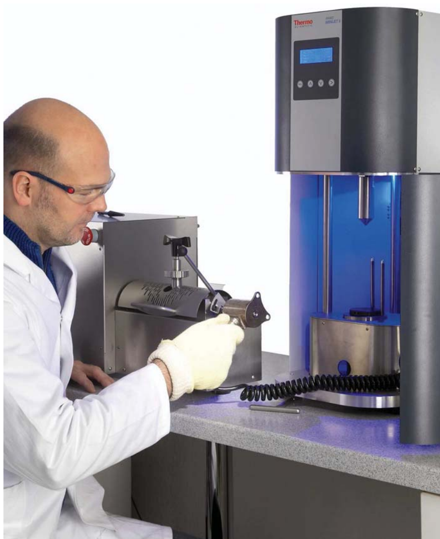
Filling the injection moulder test sample die from the HAAKE MiniCTW
