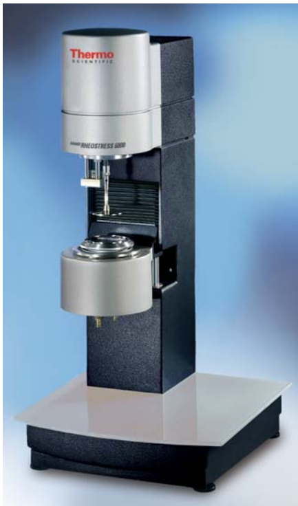
Controlled stress rheometers such as the HAAKE RheoStress provide the data to determine flow, viscosity and yield point as well as elasticity dominated properties such as die swell, ribbing and gel strength
