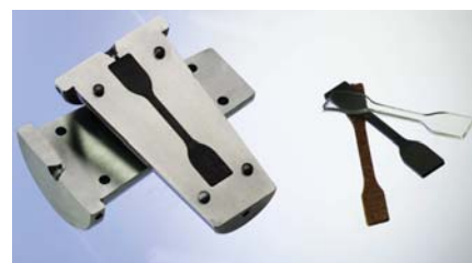
Picture 1: Mould and test specimens for tensile test
