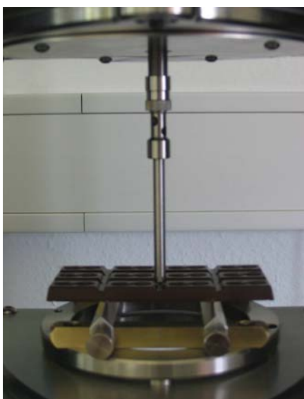
HAAKE MARS with bending and breaking tool for measuring the breaking behaviour of chocolate
