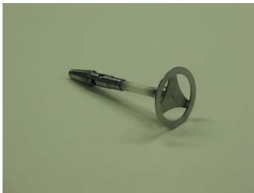
Figure 2: Newly designed ring rotor (order number 222-1789)
