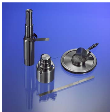
Fig. 1: Sample loading tool for cone/plate – measuring geometries consisting of forming tool (left), tool to check the geometry (middle) and strips out of stainless steel (in the front); measuring plate cover with sample loading tool (right)
