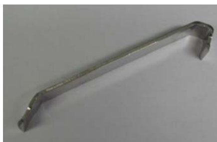
Fig. 2: Trimming tool to remove surplus material for medium and high viscous samples
