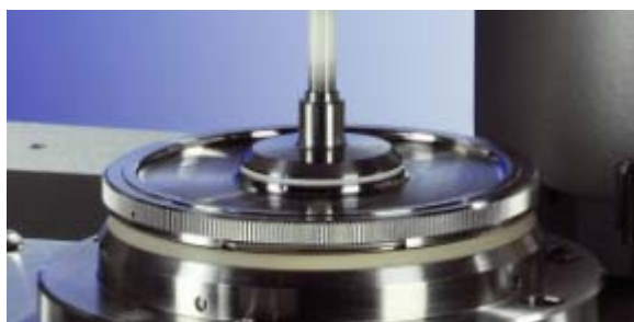
Fig. 1: Plate/Plate – measuring geometry with measuring plate cover (MPC) for optimized gap filling
