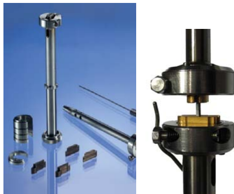
Fig. 1: Solids clamps set (left) and a sample held by the clamps (right)
