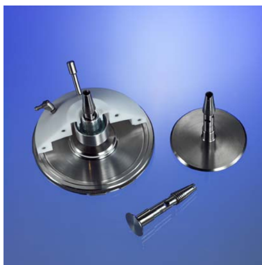
Fig. 1: Titanium geometry with measuring plate cover with same diameter for optimized gap filling; sample hood with integrated solvent trap
