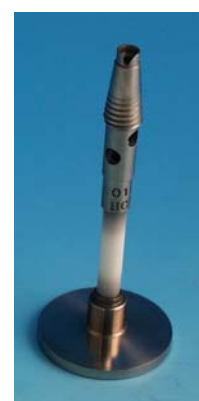
Fig. 1: Titanium geometry with measuring plate cover with same diameter for optimized gap filling; sample hood with integrated solvent trap
