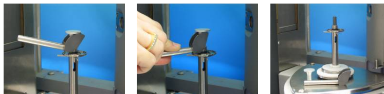
Fig. 2 Removing of a disposable plate from a shaft: removal tool positioned on the lower shaft (left). Handling of the removal tool (middle). Disassembled disposable geometry (left)
