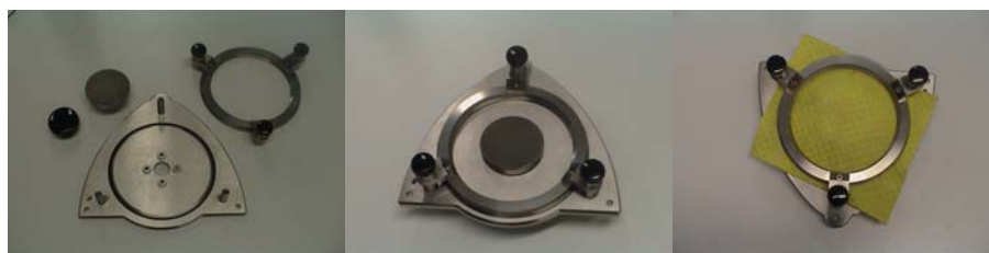
Fig. 1: Components of the textile support fixture: exchangeable measuring plate with fixing screw, lower adapter plate with centering pins, and clamp ring with screws to fix the samples (left), textile support fixture assembled without (middle) and with sample (right).
