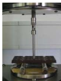
Fig. 1: Test equipment to measure the breaking behaviour of a chocolate bar
