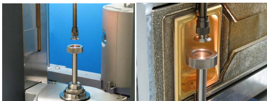
Fig. 1: UV curing cell integrated in CTC for HAAKE MARS
