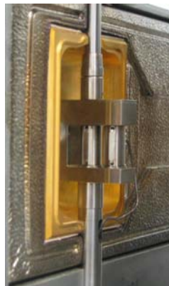
Fig. 1: SER tool integrated in Controlled Test Chamber
