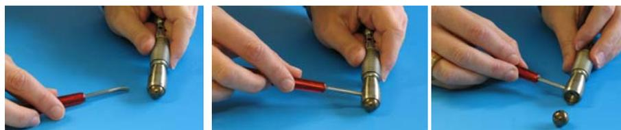
Fig. 4 – 6: Easy and user-friendly remove of a used bearing ball from the upper holder of the tribology cell
