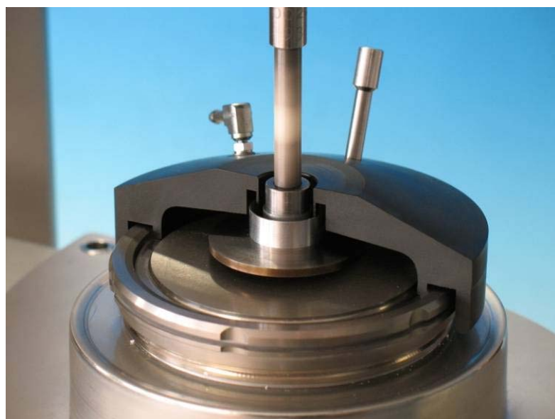
Fig. 2: Temperature module with plate / plate measuring geometry and one half of a sample hood (made of POM: 222-1903) with integrated solvent trap
