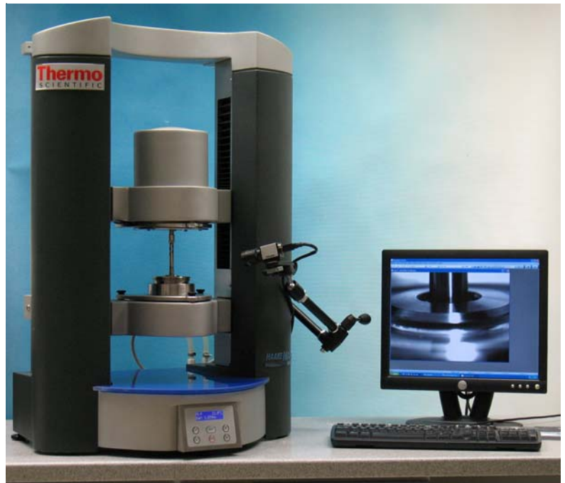
Fig. 1: Thermo Scientific HAAKE MARS III with mounted camera adjusted to the front side
