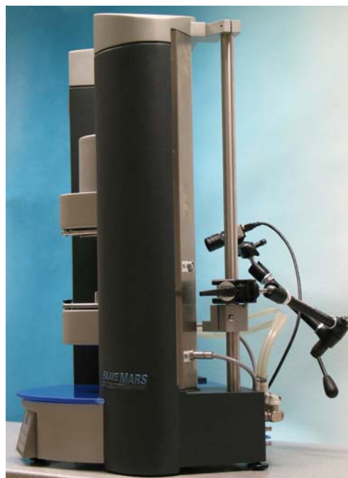
Fig. 2: Thermo Scientific HAAKE MARS III with mounted camera to the rear side
