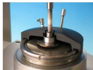
Fig. 1: Sample hood made of POM (222-1903): showing one half only
