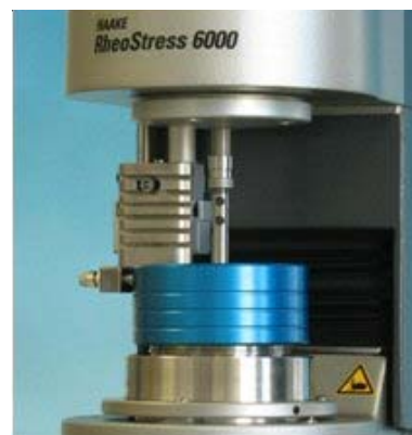
Fig. 2: Insulated sample hood TM-IN-H mounted on a HAAKE RheoStress 6000 (222-1964)
