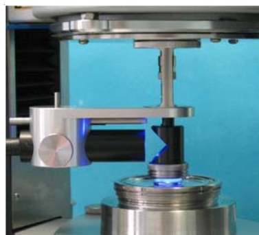
Fig. 2: Measuring geometry and adapter for mounting and adjusting the collimator and light guide
