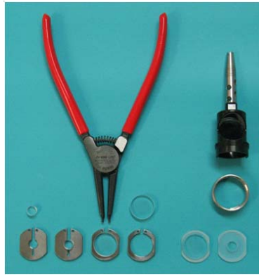
Fig. 3: Accessories for the UV module: Tool for spreading the glass plate clamps, clamps for circular glass plates with diameters of 8 and 20 mm, 8 and 20 mm circular glass plates with and without clamps, the one piece 8 and 20 mm plates glass, upper measuring geometry
