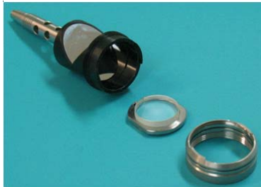
Fig. 4: Upper measuring geometry consisting of a shaft with integrated mirror and a screw holder ring for mounting the exchangeable quartz glass plate, here with a circular quartz glass plate with 20 mm and steel clamp ring
