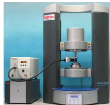
Fig. 1: HAAKE MARS III configuration for UV curing measurements incl. temperature control
