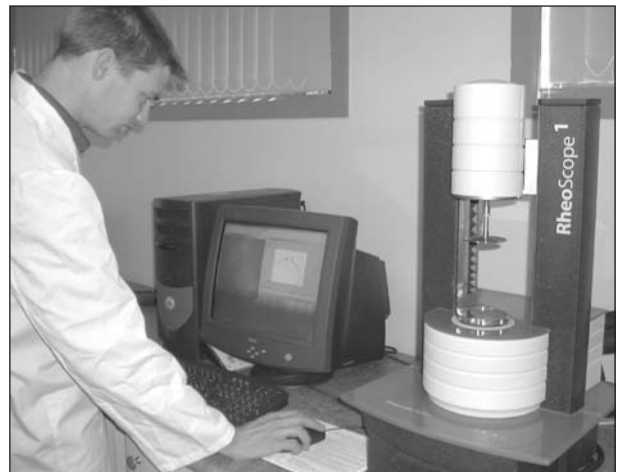
Tim Kealy setting the zero point on the RheoScope
