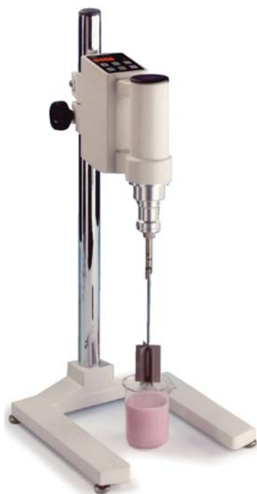
Thermo Scientific HAAKE Viscotester 550 - controlled rate viscometer
